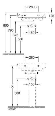
Note: All dimensions are in millimetres and are subject to normal manufacturing variations. Always use the physical product measurements for cut-outs and rough-ins as the technical details shown may differ from the actual product. Use acetic cured silicone sealant. Do not use epoxy type adhesives. Clean with damp cloth. Do not use abrasive cleaners, liquids or pastes.
