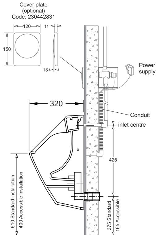
Note: Flush pipe must be vertical until the 90° bend at the urinal entry. There must be no other bends than this.
