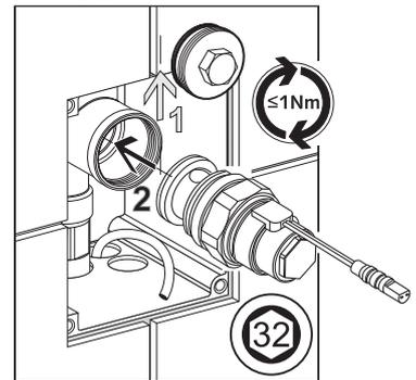
2. Remove the white plastic blanking plug from the solenoid cavity
