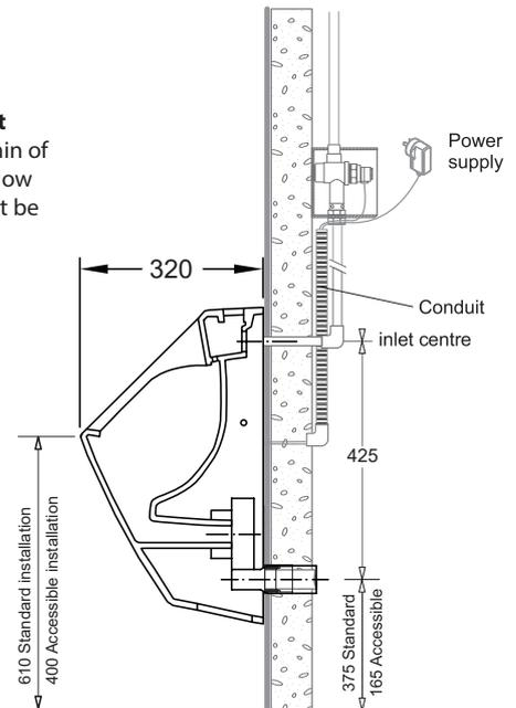
Note: Flush pipe must be vertical until the 90° bend at the urinal entry. There must be no other bends than this.
