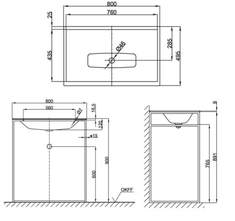
Note: All dimensions are in millimetres and are subject to normal manufacturing variations. Always use the physical product measurements for cut-outs and rough-ins as the technical details shown may differ from the actual product. Use acetic cured silicone sealant. Do not use epoxy type adhesives. Clean with damp cloth. Do not use abrasive cleaners, liquids or pastes.
