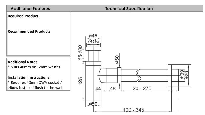
Note: All dimensions are in millimetres and are subject to normal manufacturing variations. Always use the physical product measurements for cut-outs and rough-ins as the technical details shown may differ from the actual product. Use acetic cured silicone sealant. Do not use epoxy type adhesives. Clean with damp cloth. Do not use abrasive cleaners, liquids or pastes.
