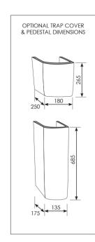
Note: All dimensions are in millimetres and are subject to normal manufacturing variations. Always use the physical product measurements for cut-outs and rough-ins as the technical details shown may differ from the actual product. Use acetic cured silicone sealant. Do not use epoxy type adhesives. Clean with damp cloth. Do not use abrasive cleaners, liquids or pastes.
