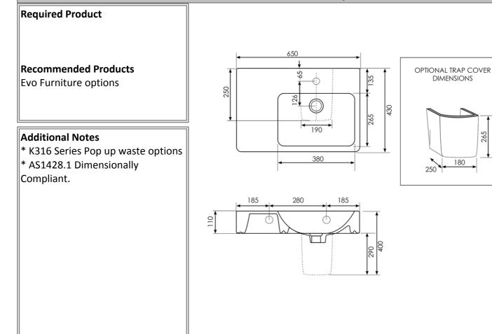
Note: All dimensions are in millimetres and are subject to normal manufacturing variations. Always use the physical product measurements for cut-outs and rough-ins as the technical details shown may differ from the actual product. Use acetic cured silicone sealant. Do not use epoxy type adhesives. Clean with damp cloth. Do not use abrasive cleaners, liquids or pastes.
