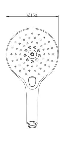
Note: All dimensions are in millimetres and are subject to normal manufacturing variations. Always use the physical product measurements for cut-outs and rough-ins as the technical details shown may differ from the actual product. Use acetic cured silicone sealant. Do not use epoxy type adhesives. Clean with damp cloth. Do not use abrasive cleaners, liquids or pastes.
