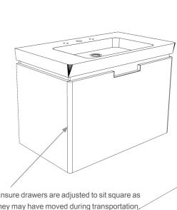
Ensure drawers are adjusted to sit square as they may have moved during transportation, Ensure runners are locked in place.
