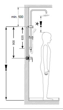
\*Water Entry Point: Recommended installation height is between 1700-1900mm from the finished shower floor.
