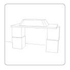
Please inspect the alignment of the under-counter basin to the basin cut out in the stone top from underneath and ensure the alignment is even all the way around.
