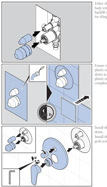
Either sheet around the mixer body with fibre cement sheeting or backfill the exposed channels ready for tiling.
