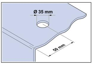
Where the mixer is going into a stone or laminate top, cut a 35mm Ø hole.
