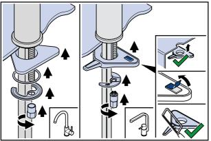
Fit the rubber gasket, holder and fixing plate assembly into position under the sink/bench top. The holder is not required for solid bench tops. Tighten the nut assembly and then tension the screws.
