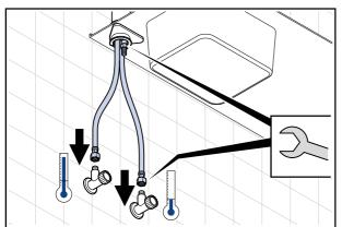
Make sure the hoses are connected to the correct hot and cold water feed.
