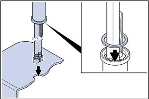
Feed the two hoses through the hole in the sink or bench top.
