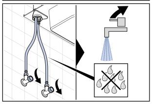
Open the stop valves (not included in scope of supply), flush the lines, then close the mixer lever and check there are no leakages.
