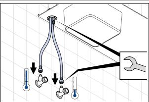
Make sure the hoses are connected to the correct hot and cold water feed and then tighten the nut.
