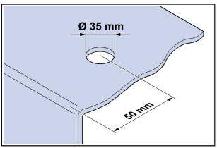
Where the mixer is going into a stone or laminate top, cut a 35mm Ø hole.
