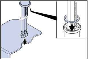
Feed the two hoses through the hole in the basin or bench top and attach to the basin mixer.
