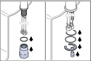
Fit the rubber gasket and fixing plate into position under the basin / bench top, fasten with the nut.
