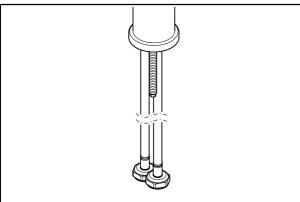
Install the allthread screw into the bottom of the basin mixer.
