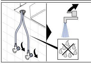
Open stop valves (not included in supply), flush the lines, then close the mixer lever and check there are no leakages.
