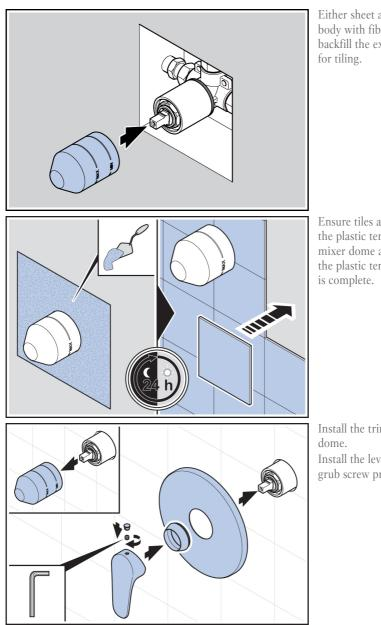
Either sheet around the mixer body with fibre cement sheeting or backfill the exposed channels ready for tiling.
