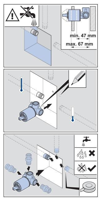
Based on the size of the body and the wall type, either secure it to the noggins or embed it into the wall at an approximate height of 1100 mm.
