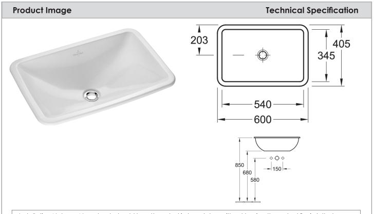
Installation Notes:  $\Box$  No cut-outs should be attempted in bench top without having the actual Basin/s that are going to be installed.  $\Box$  Only Silicon based adhesives should be used, not epoxy resins.  $\Box$  Overflow hole should be positioned closest to the front of the cabinet.
